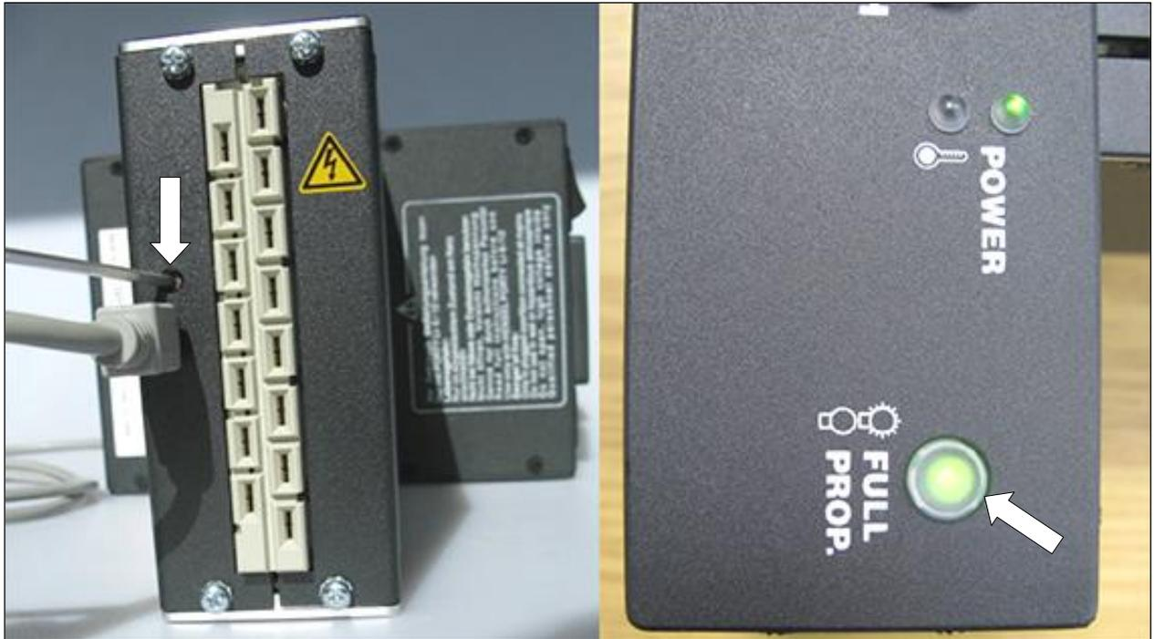
1) Connect the AC power supply drawer via the USB socket to your computer before switching the unit on.
